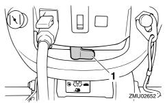
1. "OPEN" position for the portable tank
